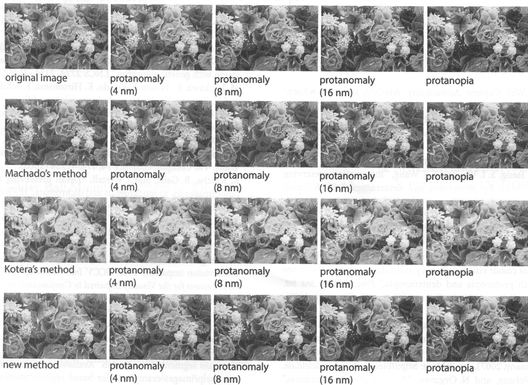
Figure 9. The daltonization results for protanopia and protanomaly obtained with Machado's, Kotera's and the new method for a complex natural image with large color gamut.
